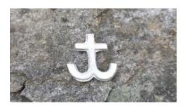
Heat the tin over a camping stove until it becomes liquid. Then pour into the prepared mold. After cooling, sand the pewter figure with files until it fits.
