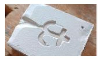
First of all, you need a mold into which you can pour the tin. This must be two parts that fit together. There are molds made of metal, plastic or clay. The molds are cleaned with powder before casting.
