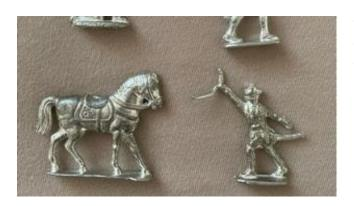
Then press the figure out of the mold and cut away the excess tin. The figure can still be finished with files and sandpaper.
