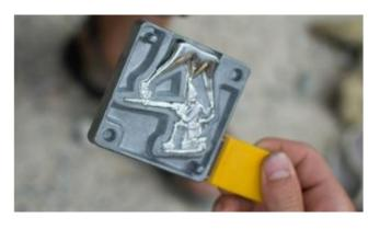
Allow the pewter to cool in the mold until it is cool at the pouring point. (feel with your finger) As soon as the pewter is cool, you can loosen the screw clamp, put the pieces of wood to one side and open the mold.
