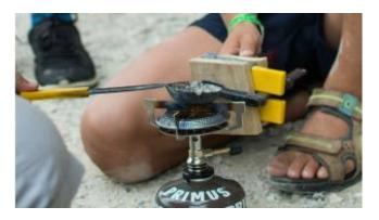
The molds are then pressed together between two pieces of wood using a screw clamp. Meanwhile, the pewter is heated in a small pan on a camping stove until it melts. As soon as the mold and pewter are ready, the liquid pewter can be poured into the mold until the mold is full.
