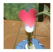
The copper heart is annealed in the flame of the Bunsen burner
