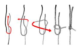
The sheet hitch is a suitable knot to connect unequal thicknesses. It is related to the Samaritan and the bowline.
